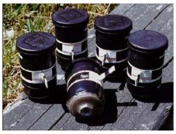
Figure 1. Pinhole camera made from a film canister
